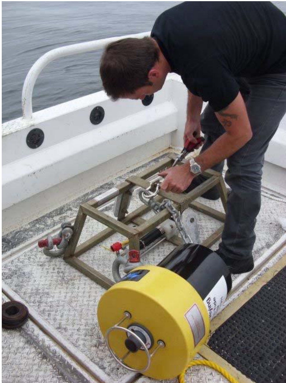
Figure 3.0-1 Attaching Acoustic Release Buoy to Submersible Tide Gauge
